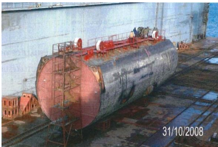
Figure 1 3-compartment reactor unit formulated and temporarily set on the floating dock FD-90 (North Eastern Regional Center)
