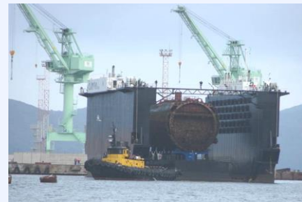
Placing an “3-RCU” on a slipway pad
